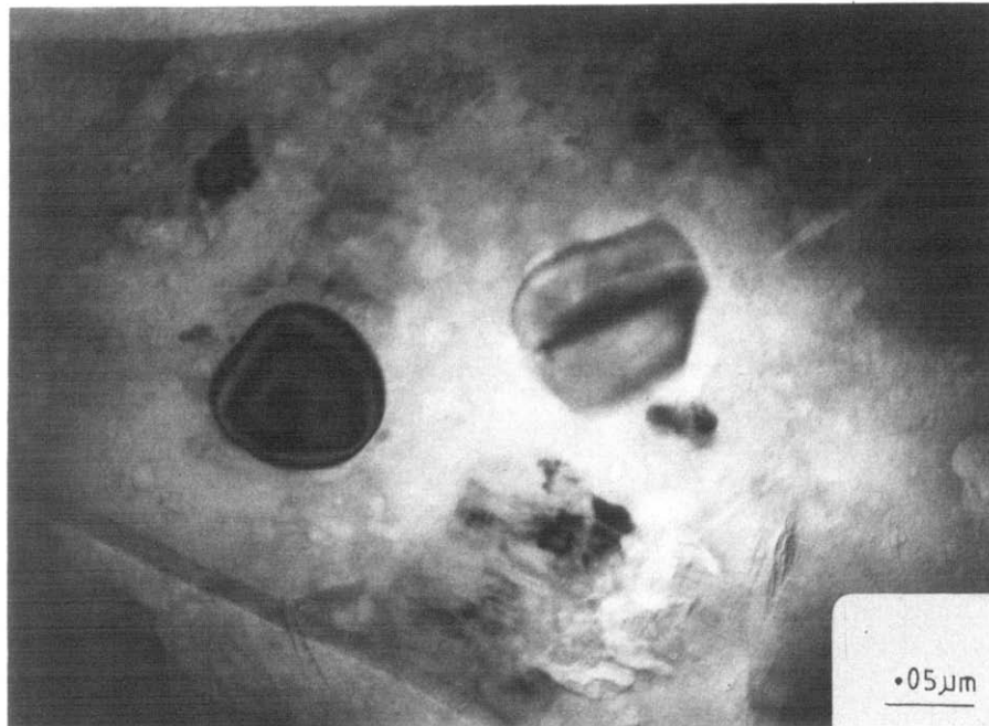
Fig. 7. TEM micrograph showing nucleation of alpha-silicon nitride on graphite.
